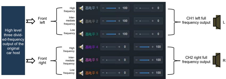
Example 3: High level active three divided-frequency mixing input, stereo full frequency output of the original car host.
