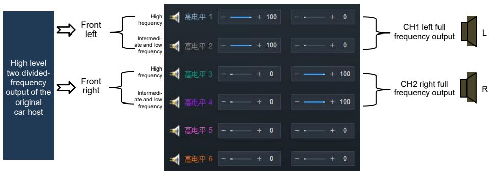
Example 3: High level active three divided-frequency mixing input, stereo full frequency output of the original car host.
